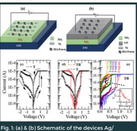
Fig. 1: (a) & (b) Schematic of the devices Ag/ BSA/TiO2/FTO (TB) & Ag/BSA/GO/TiO2/FTO (TGB) respectively. (c – d) I – V characteristics, which demonstrates that these devices are sensitive to the detection of BSA.
